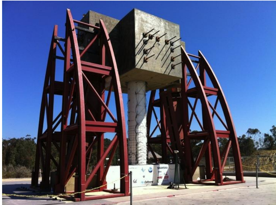
Full-scale 1D tests of circular column - J. Restrepo, PI (PEER, Caltrans, UNR, FHWA, NEEScomm & NSF)
