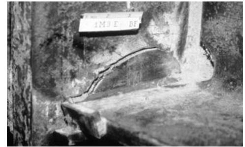
Column Fracture in Beam Column Testing (courtesy of M. Engelhart)
